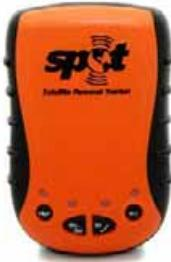
It can be used as a personal locator beacon to call for emergency from anywhere with a press of a button. **No cell phone coverage is needed.** Emergency services will get an immediate notification with GPS coordinates. This can be a life saver in case of a bad landout or a crash, which may happen where no cell phone service is available.
